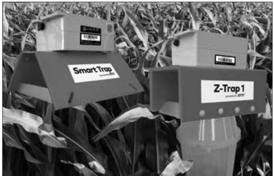
Automated pheromone traps can monitor WBC populations. The Z-trap on the right uses a bucket trap to collect WBC moths.
